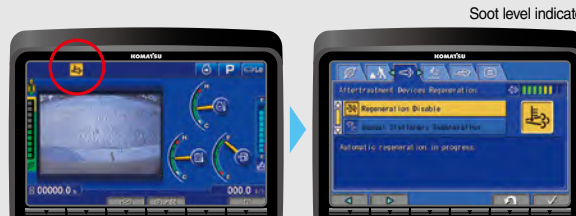
Aftertreatment device regeneration screen
