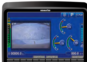
Rear view image on monitor
